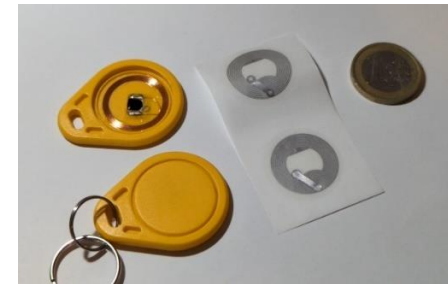
Figure A3: MIFARE Classic droplet (left) and Ultralight sticker (right)
