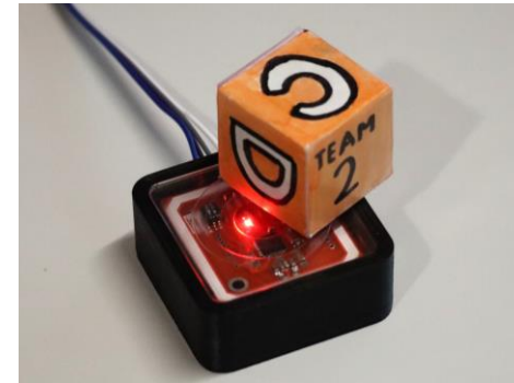
Figure 7: RFID reader custom 3D printed design
